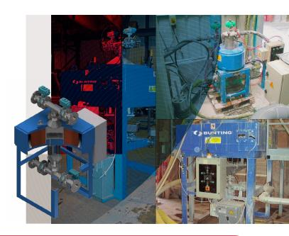
Filters are fitted with an auto backflush system on a timed cycle to enhance performance and to prevent clogging. This feature proves to be particularly successful where superior quality ceramics are required, outperforming competitor units.
